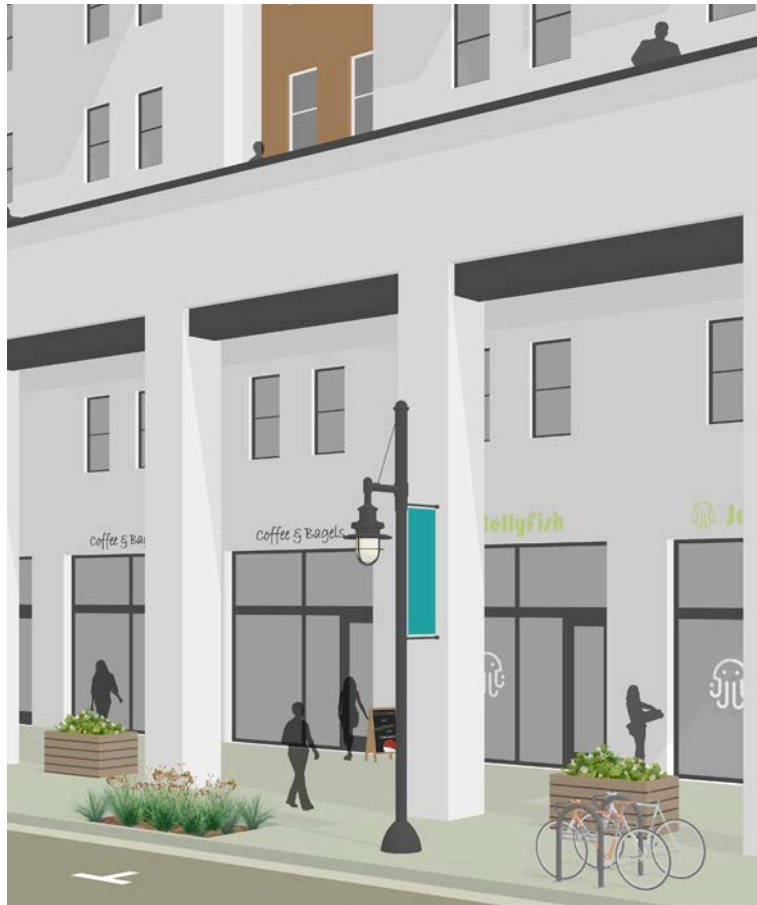
5g. Design retail shopfronts with relatively large, transparent first floor windows tall enough to provide adequate view into ground-floor spaces. Retail shopfront glass should be transparent.
