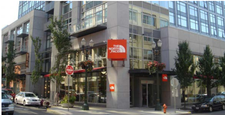
8a. "Hold the building corner" by placing a building façade within the build-to area at the block corner for a distance of at least 50 feet from the corner, and by providing distinctive building elements or other treatments.
