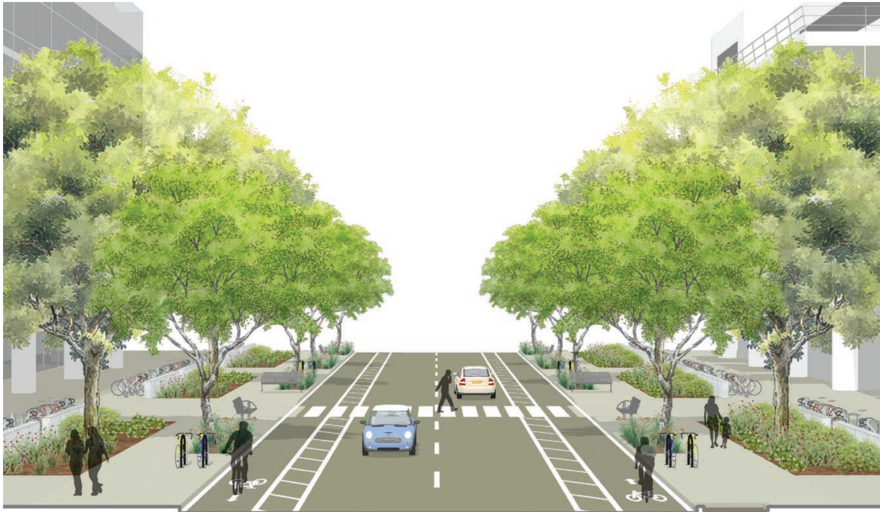
Figure 32: Access Street: Potential Cross Section
