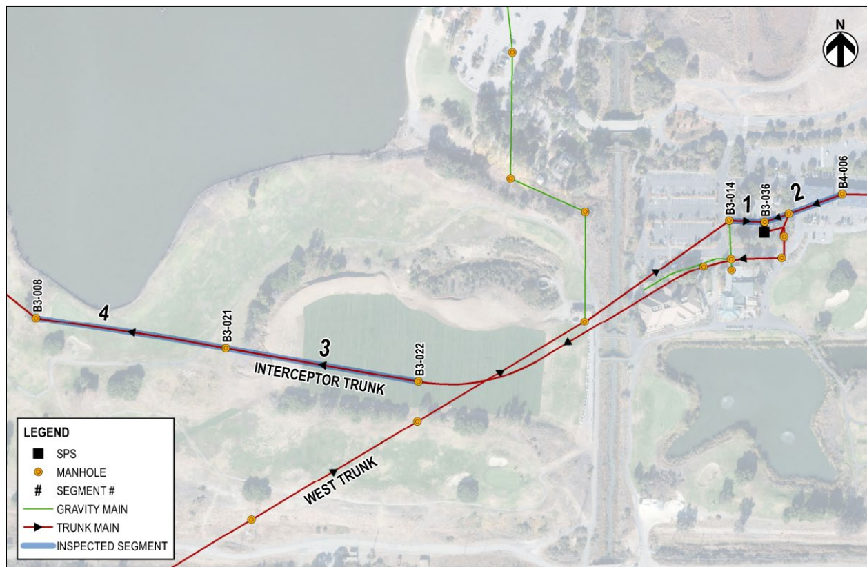
Figure 4-3: SPS Vicinity Piping Segments Inspected
