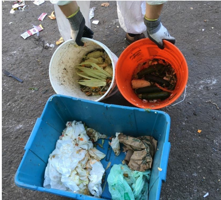
Organics load sorted into Inedible Food Scraps, Edible Food Scraps, Paper Towels & Tissues, Compostable Paper and Compostable Plastic Bags
