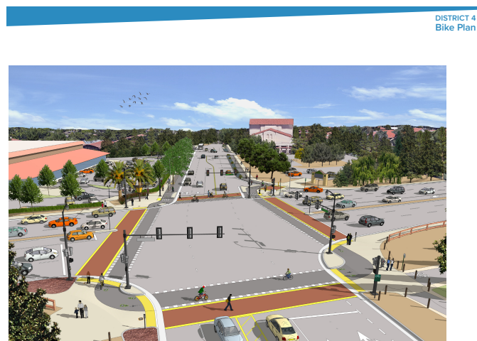
The City of Palo Alto and Stanford University have worked together to develop a protected intersection on El Camino Real (State Route 82) and Embarcadero Road/Calver Street. The design removes several slip lanes, provides a clear path for bicyclists through the intersection and connects to trails on either side of El Camino Real. Rendering courtesy of the City of Palo Alto and Calander Associates.
