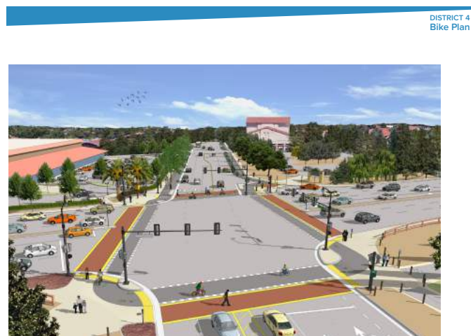
The City of Palo Alto and Stanford University have worked together to develop a protected intersection on El Camino Real (State Route 82) and Embarcadero Road/Calver Street. The design removes several slip lanes, provides a clear path for bicyclists through the intersection and connects to trails on either side of El Camino Real. Rendering courtesy of the City of Palo Alto and Calender Associates.
